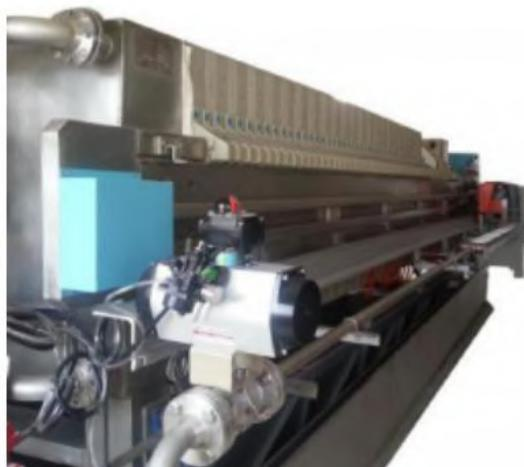
Hongmao filter press is composed of filter plate, frame, cylinder, automatic plate shifting, electric cabinet, hydraulic station and drip tray. There are different kinds of filter press used in different production field, for example: mechanical frame filter press, manual filter press, membrane filter press, chamber filter press, hydraulic frame filter press, etc.
