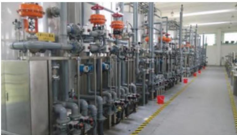
Hongmao automatic intelligent ion exchange system, using valve array control, desalting (decoloring), regeneration, washing at the same time, intelligent control, one-button start, online monitoring of various indicators.
