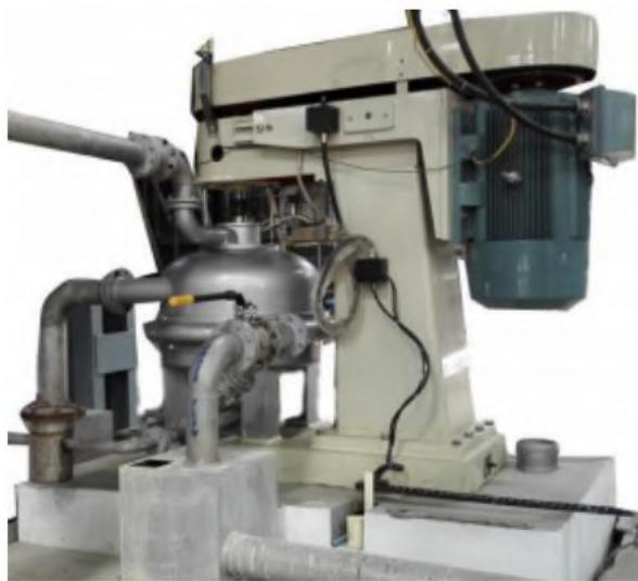
In the starch separation process, Hongmao disc separator produces very high centrifugal force due to high speed rotation, which improves the separation efficiency and maximizes the production efficiency. It has the advantages of all kinds of separator, small vibration, large handling capacity and stable operation. It is mainly used in pre-concentration of starch, separation of starch and gluten, concentration of gluten (protein) and clarification of water in the process.
