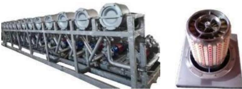
The starch milk and the washing water go through the washing system in a countercurrent way. The washing system usually consists of 6-12 grades. Each stage contains a number of cyclone tubes which are housed in the housing of the cyclone separator and operate in parallel.
