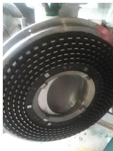
HM-DM-P series degerm mill is a larger coarse crushing equipment in wet corn starch production process. It is suitable for corn to break up once or twice after steeping, so that the germ, skin and endosperm are separated from each other.
